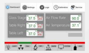
Color Touch Screen PLC Control panel with data log and Alarm functions
