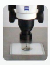
Flush mount Glass Stage Warmer with 3 mm clearance and temperature accuracy  $\pm 0.5^{\circ}$ C
